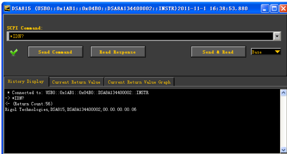
Figure 3-3 Write and Read Commands via USB
