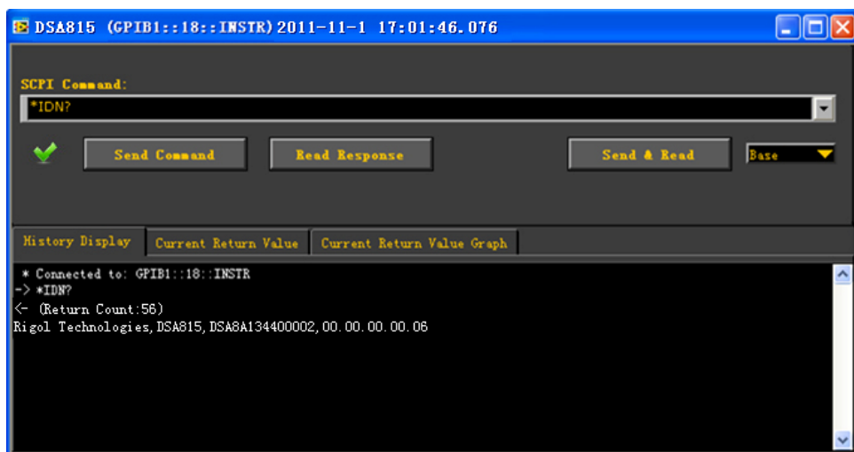
Figure 3-10 Write and Read Commands via GPIB
